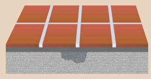
Localised deep holes may result in a bed thickness that exceeds the specification for a thin-bed adhesive.
