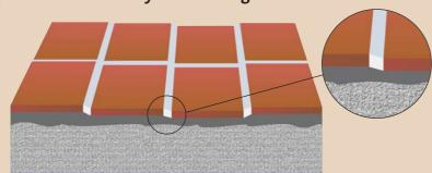
A serrated adhesive spreading trowel, when used at a constant angle, enables the even distribution of adhesive onto the substrate. If the tiles are all bedded with a similar force they should be at the same height with only minimal unevenness. However, if the substrate is not level, this is much more difficult to achieve and there is more chance that some edges will be standing proud.
