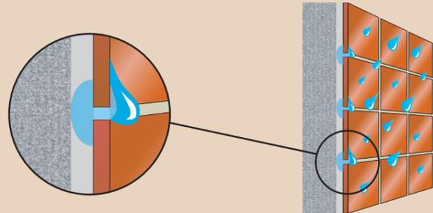
Most cement-based products including grouts and adhesives are porous to some extent.
