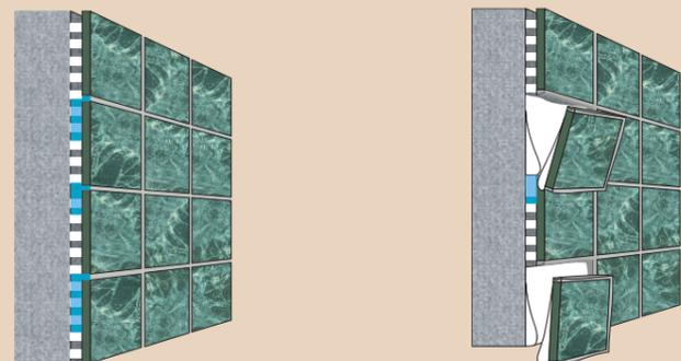
Most ready-mixed adhesives are water-based. They set by allowing the water to dry out and form a strong hard bond.
