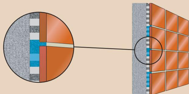
Voids left in the adhesive layer after bedding the tiles will allow any water that penetrates the grout or sealant to gather.
