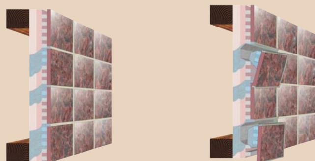
Some substrates, particularly gypsum plaster and plasterboard, have very little strength when wet.
