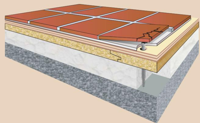
When a floating floor is over-boarded to add rigidity, the extra board has to be securely attached to the original boards. If nails are used, the constant movement of the floor can cause them to work loose, press on the underside of the tile and cause cracks to form. If the screws/nails used are too long they can bottom out on a rigid surface under the floating floor and create a column, over which tiles will crack.
