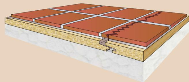
If a joint between wooden boards of a floating floor is not correctly located or fixed, it will be susceptible to highly localised movement which will crack the tile along the joint.
