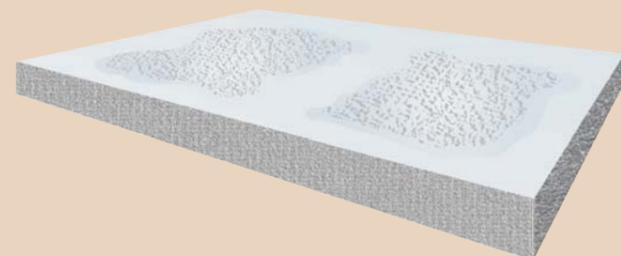
As anhydrite cures, a weak layer of laitance is formed on the surface.
