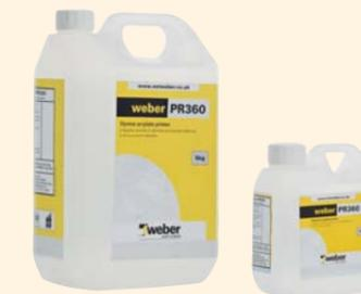
Seal the floor with **weber PR360** repeatedly until no more is absorbed and allow the primer to dry before tiling.
