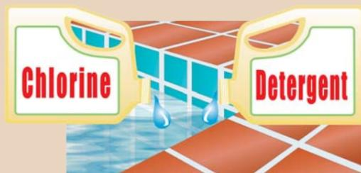
Chemicals added to the pool water tend to degrade cement-based grouts. This is minimised if they are maintained at the ideal levels but the choice of grout and its chemical resistance are important factors for the durability of the installation.
