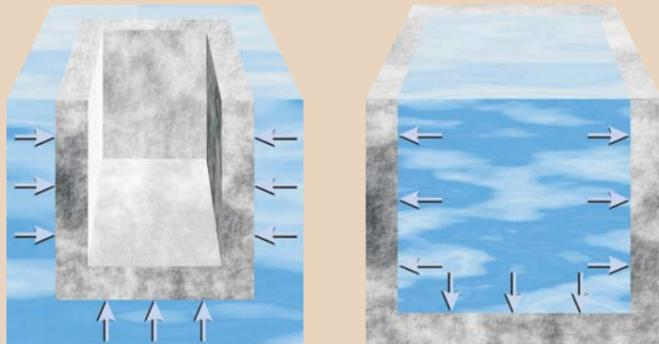
Concrete is naturally porous and should not be considered to be a water-tight structure. Water will slowly seep through tiny pores in the concrete and this is exacerbated when the water is under pressure.
