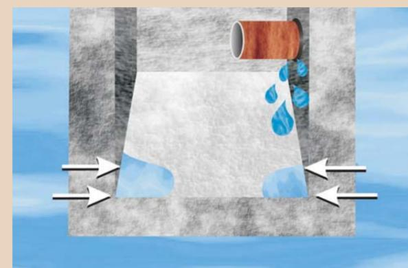
Internal corners are subject to large stresses and this often leads to cracking allowing water ingress.
