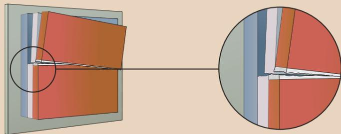
When the surface is very smooth this grip is much weaker resulting in tiles de-bonding.
