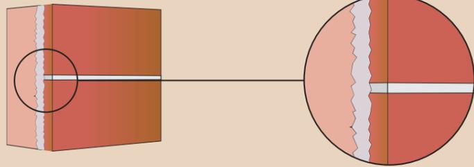
Standard cement-based adhesives rely on a mechanical keying action to bond onto the substrate. The wet cement engages physically with small irregularities, pores etc in the surface and uses this to form a strong bond.
