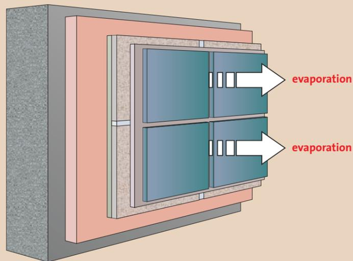
Ready-mixed adhesives are dispersions of polymers and inert fillers in water and do not gain strength until the majority of the water has dried out. With large tiles on impervious surfaces, this can take weeks.
