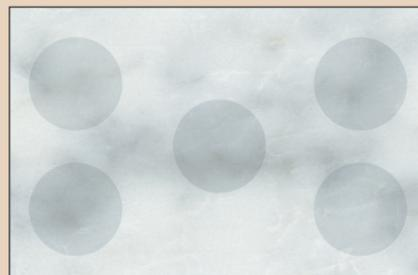
Some tiles and natural stones (e.g. limestone and marble) will show a shadow on the face where the adhesive is in contact behind. Voids will be visible from the front of the tiles.
